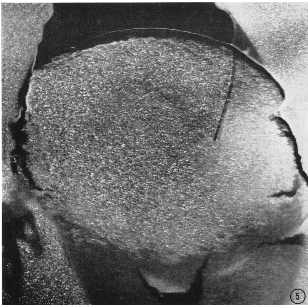
FIGURE 5 Dark-field electron micrograph of a chromium-shadowed human red blood cell. This image was produced by moving the objective aperture off-axis until it transmitted a portion of the (111) Debye-Scherrer ring. Individual microcrystals which are oriented so that they satisfy the appropriate Bragg condition are thereby imaged as bright spots. Note that the crystal size formed over the cell surface is the same as that formed over the (mica) substrate.
